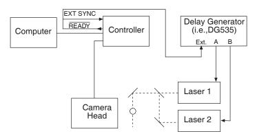
Figure 57. Another Hardware Setup for an IEC Measurement
